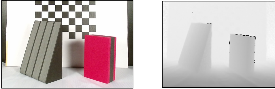
FIGURE 5 (On the left) an RGB image and (on the right) a depth map captured with a ToF camera before image rectification. Lighter pixel color means that the corresponding point in scene space is farther from the camera.
