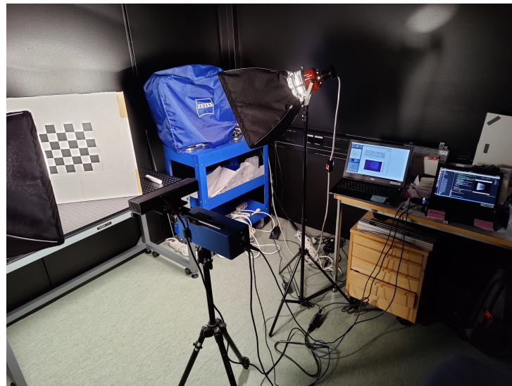
Figure 5. The experimental calibration setup with the hyperspectral camera, Kinect, halogen diffusers, and realignable checkerboard calibration pattern.
