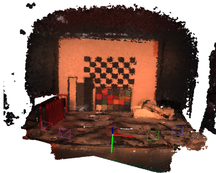
Figure 8. The fully registered point cloud with pseudo RGB coloring and the visualizations of camera capture viewpoints.
