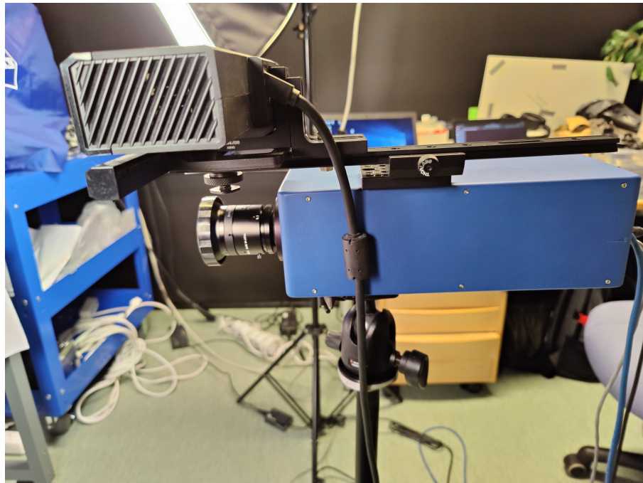
Figure 1. The prototype FPI hyperspectral camera ( below ) and the Kinect ( on top ) used in the research.
