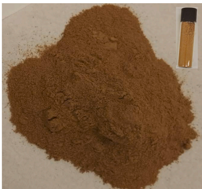
Fig. 1. Pictorial representation of lateritic soil with characteristic reddish-brown color. Inset is an example of how the soil sample used in this study was stored in an airtight vial for characterization.
