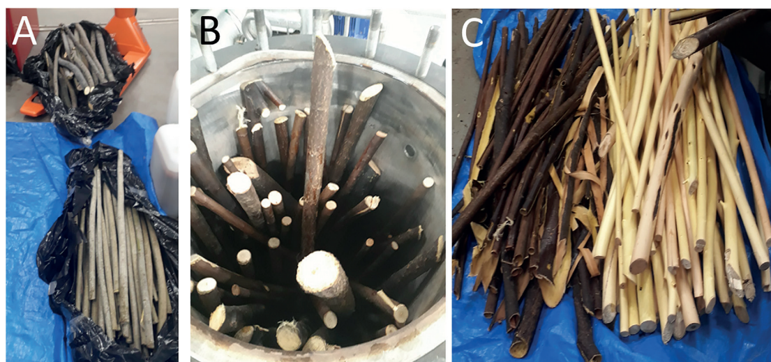
FIGURE 1 | Original willow samples (A), combined willow sticks in reactor (B), and steam-treated bark and woody material (C).
