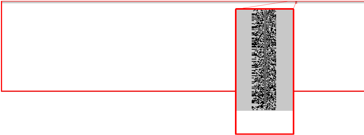
Fig. 6. Bitmap obtained from a readback operation after a run of a CNN Int 16 version. Each pixel represents a bit; each bit that was identified with an error appears in black. The red lines are used to limit the region. The grey zone represents the memory usage. Zoom-in is added to increase the visibility of the block event.
