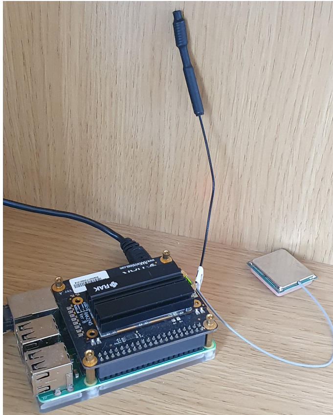
Figure 5.7: RAK LoRaWAN gateway
