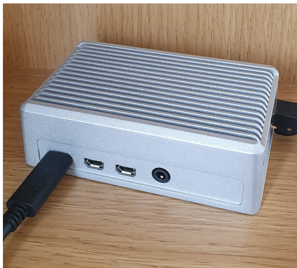
Figure 5.8: Raspberry PI server for data processing
