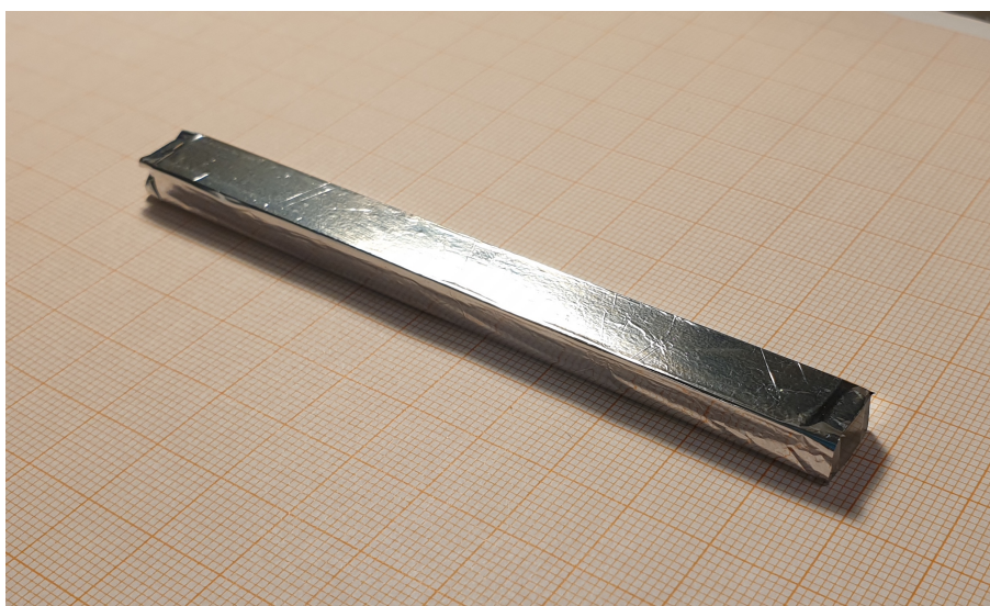
Figure 23. A bar of scintillator plastic coated in white paint, with a layer of ZnS on top, fully wrapped in mylar. This is a fully finished scintillator element ready to be used in the finished prototype.
