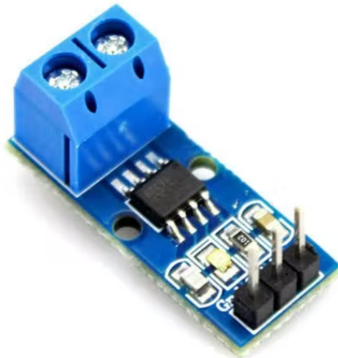
Figure 10. The ACS 712 current sensor used in monitoring the supply currents for the ADA4870 operational amplifiers. The supply voltage of 5 V DC is connected to the left and right side pins where the output signal is got from the central pin. The output signal is delivered through the rack case into the Wago TM I/O system for digitization. Figure from [31].
