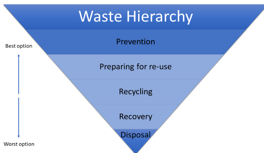
Figure 1. Waste hierarchy. Adapted from European Commission Waste Framework Directive (European Commission, n.d.).
