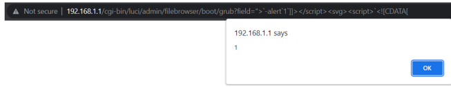
Fig. 8. Evaluation on RPi3 with OpenWrt (device): Screenshot depicting XSS in OpenWrt's LuCI Web interface running on RPi3 without HALE-IoT .
