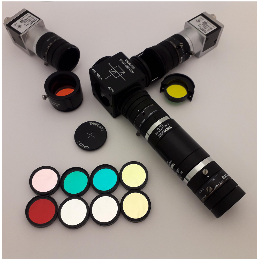
FIGURE 66 Future work consists of two monochromatic machine vision sensors, a 50:50 beam splitter, several C-mount lenses, extension tubes, tunable filter holders and adapters between the optomechanical components. The system will have ten (10) selected band-pass filters and a software to optimise the best wavelength combination target-wisely.
