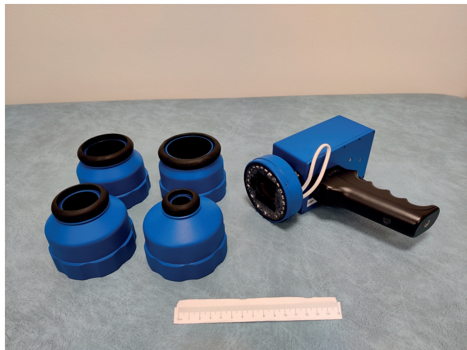
Figure 1. SICSURFIS spectral imager with integrated LED module and stray light protection cones.
