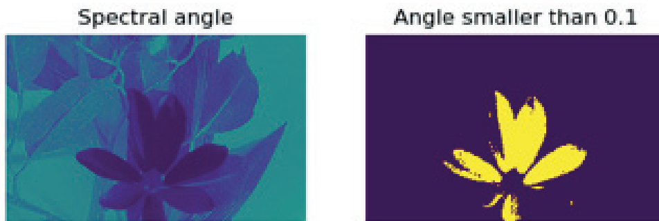
Figure 7: Spectral angle as compared to a pixel spectra from the real plant (left) and thresholded spectral angle (right).
