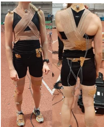
Figure 5. Experimental design. A: Capture volume. B: Subject preparation with EMG and reflective markers.
