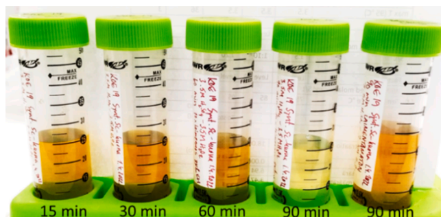
Fig. 7. Diluted (10x) 15-, 30-, 60- and 90-min samples after leaching synthetic slag with 3.5 M H 2 SO 4 + 3.5 M H 2 O 2 at 100 °C and S/L of 1:10. A sample of undiluted residual liquid is shown on the right.
