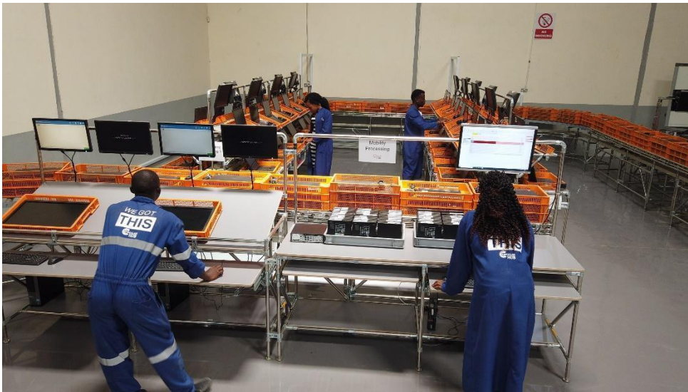
Photo 2: Checking and data wiping process at CE-HUB
