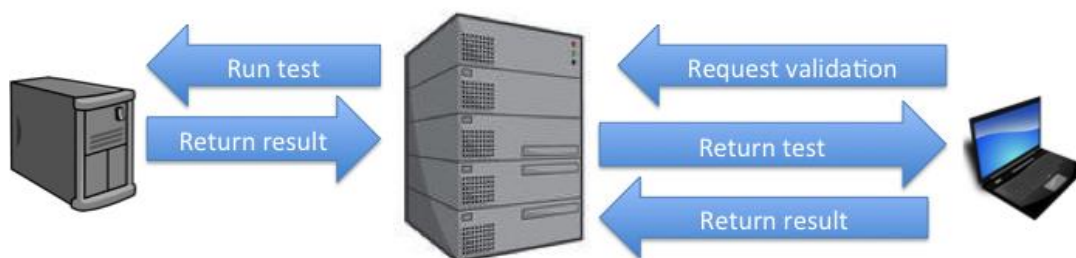
Figure 11: Naïve Verification Procedure. The remote machine (on the right) requests validation. The distributor (in the middle) generates a test and runs it on a local machine (on
