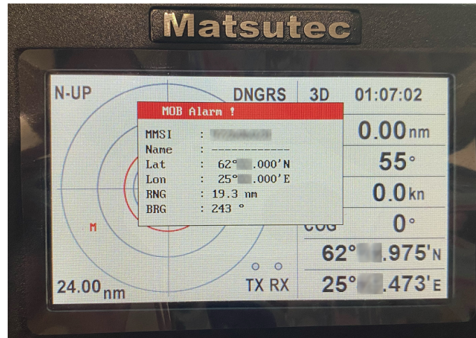
FIGURE 33 Matsutec HP-33A AIS transponder showing an MOB alert
