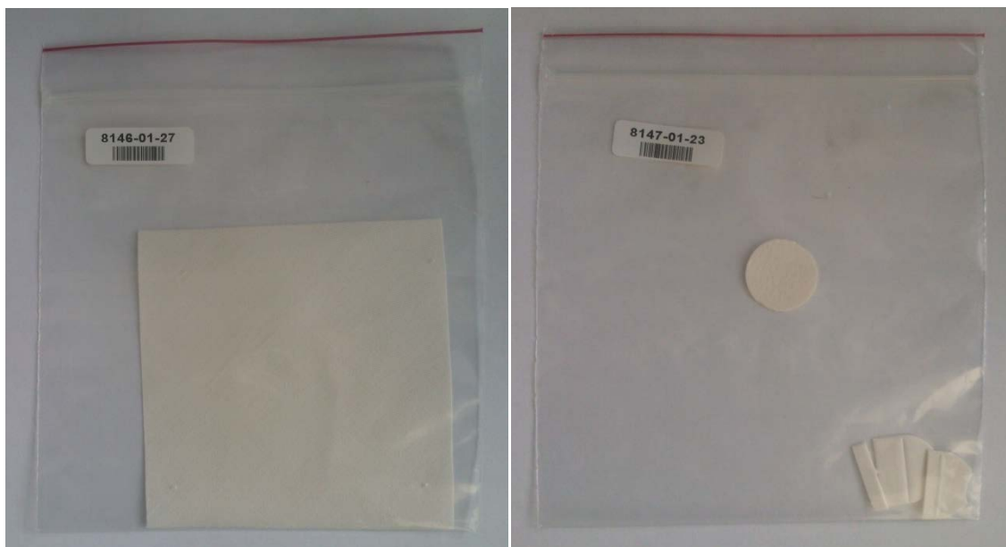
FIGURE 22. IAEA swipe samples. The two reference samples were large square-shaped swipes like sample 8146-01-27 on the left and the four unknown samples smaller round swipes like sample 8147-01-23 on the right.
