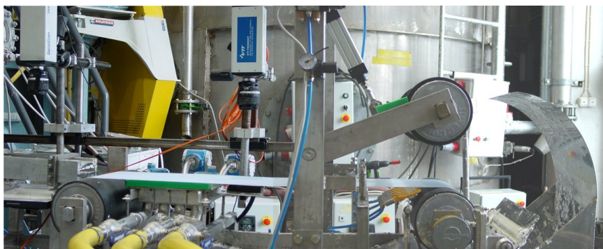
Figure 1. The pilot former for simulation of drainage, filtration, and flocculation.
