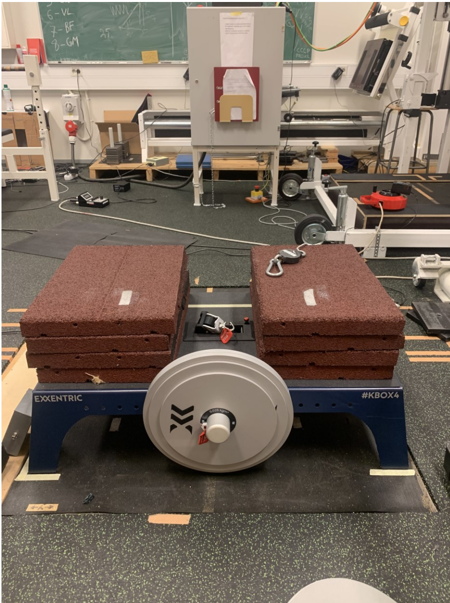
FIGURE 13. Flywheel setting. Exxentric kBox 4 Pro and their flywheels were used in this study. Elevated platforms had to be placed on top of the kBox since the pulling force meter would have otherwise gotten tangled with the flywheels. White tape marks are placed on top of the platform at the subjects desired stance width.
