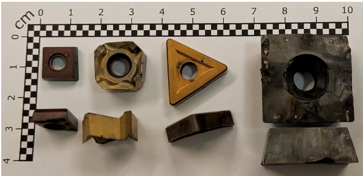
Figure 21. Four arbitrary example scrap pieces provided by Tikomet. Top and side views from each sample with a length scale in centimetres for reference. Sample numbers from left to right: 7, 13, 14 and 16. The spots visible in the pieces in the top row are the craters caused by LIBS measurements.
