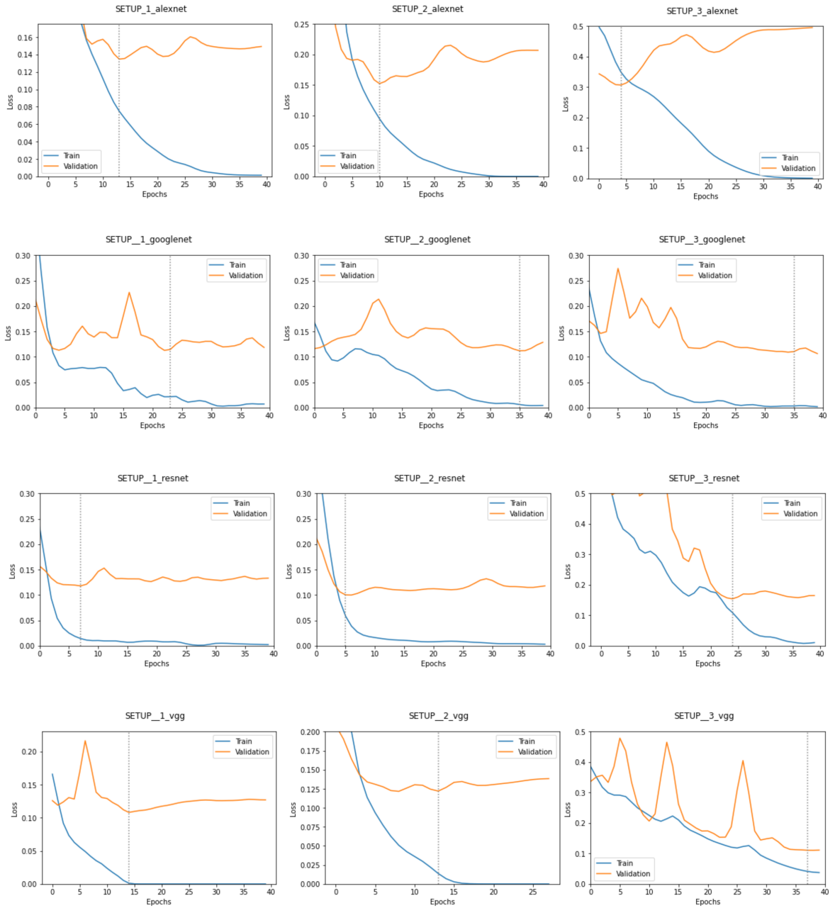
Figure 12: Training and validation losses for all setups and CNNs. Vertical line represents the point where training was stopped when training the final model.
