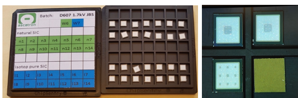
Fig. 3. Left: Box with bare die diodes, 14 natural SiC, and 14 mono-isotopic SiC. Right: Close up of 4 diodes, bottom right shows cathode/backside, the 3 others show anode/front side.
