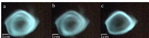
FIG. 5. (Color online) Two concentric hollow beams can be obtained with two frequency heating: (a) 14.070 GHz+11.56 GHz, (b) 14.100 GHz +11.56 GHz, and (c) 14.135 GHz+11.56 GHz. RF-power=203 W +30 W, pressure= 3.9 \times 10^{-7} mbar, and BD=-68 V.
