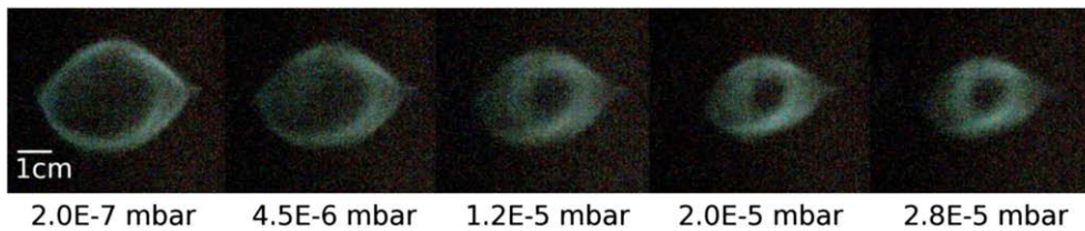
Fig. 7. The beam viewer image of \text{Ar}^{8+} with helium as feeding gas with various beam line pressures.
