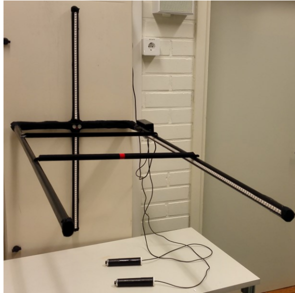
Figure 8. Custom made device for visual field and peripheral reaction speed measurements.
