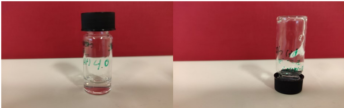
Figure 5. Preparation of HA-ADH gels at the final pH 4.0. Trial 1 did not yield a self-supporting gel but a viscous flowing solution.
