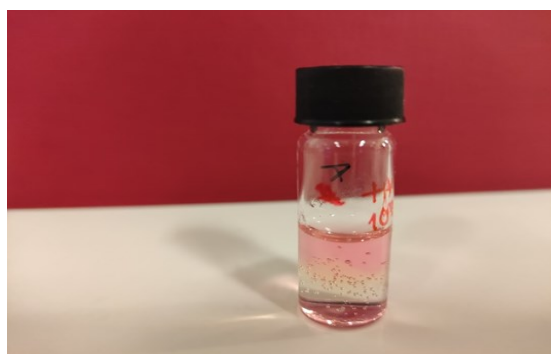
Figure 12. An HA-ADH gel after incubation in the presence of the cell culture medium. The pink colour is due to the pH indicator within the cell culture medium.
