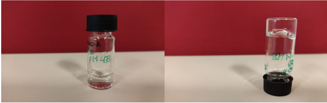
Figure 6. Preparation of HA-ADH gels at pH 4.8. Trial 2 yielded a self-supporting gel.
