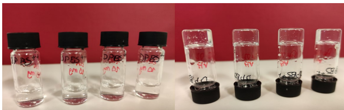
Figure 11. HA-ADH gels in DPBS ++ solution prepared by the standard gelation protocol. All the gels are self-supporting.
