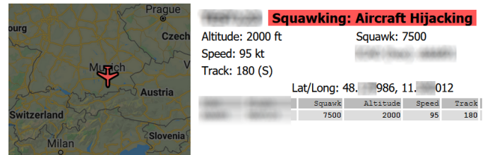
Fig. 7: Fake distress squawk code in the Dump1090 net.
