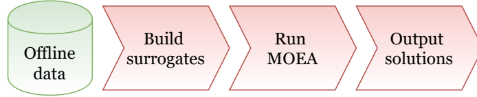
FIGURE 1 Flowchart of a generic offline data-driven multiobjective optimization approach.
