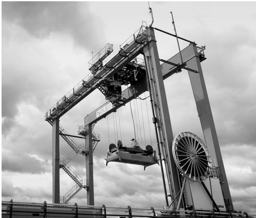
FIGURE 12. Spreader retrieving a container (Kalmar, Introducing Kalmar presentation, 2018)
