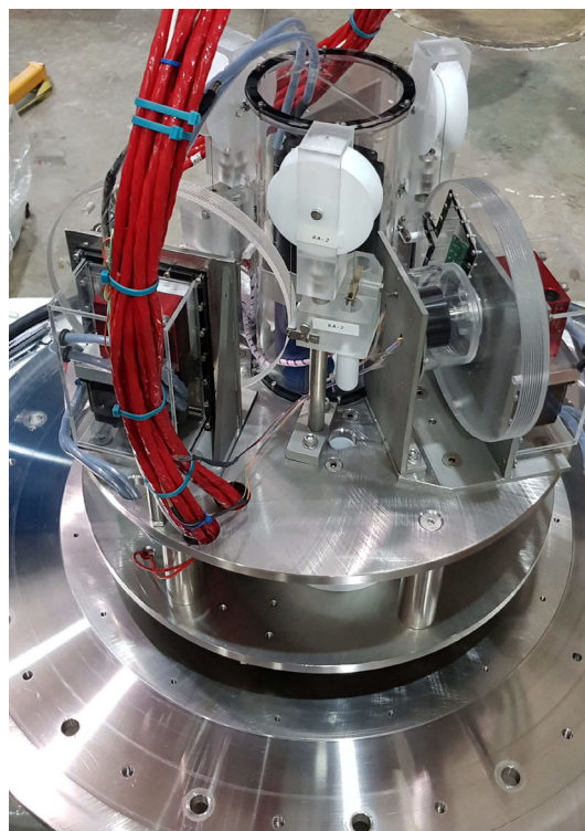
Fig. 11 The automated calibration system (ACU) with the bell jar removed. Three acrylic winches are mounted to a turntable, allowing to lower sources down into the detector through a 1-in. hole in the bottom plate
