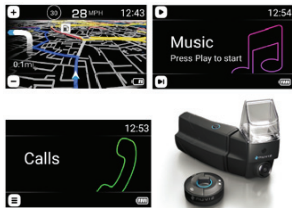
Figure 2: On top: Nuviz HUD user interfaces (navigation and music). On bottom: Nuviz HUD user interface (calls) and Nuviz HUD device with the controller. NB. During the distraction testing the controller did not have any labelling on it.
