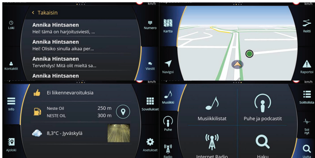
Figure 2. Views of the automotive-targeted application (Carrio). Left upper corner: email reading view, right upper corner: navigation view, left lower corner: weather condition view, and right lower: corner song searching view. The navigation view and the weather condition view were only used in the view switching task.
