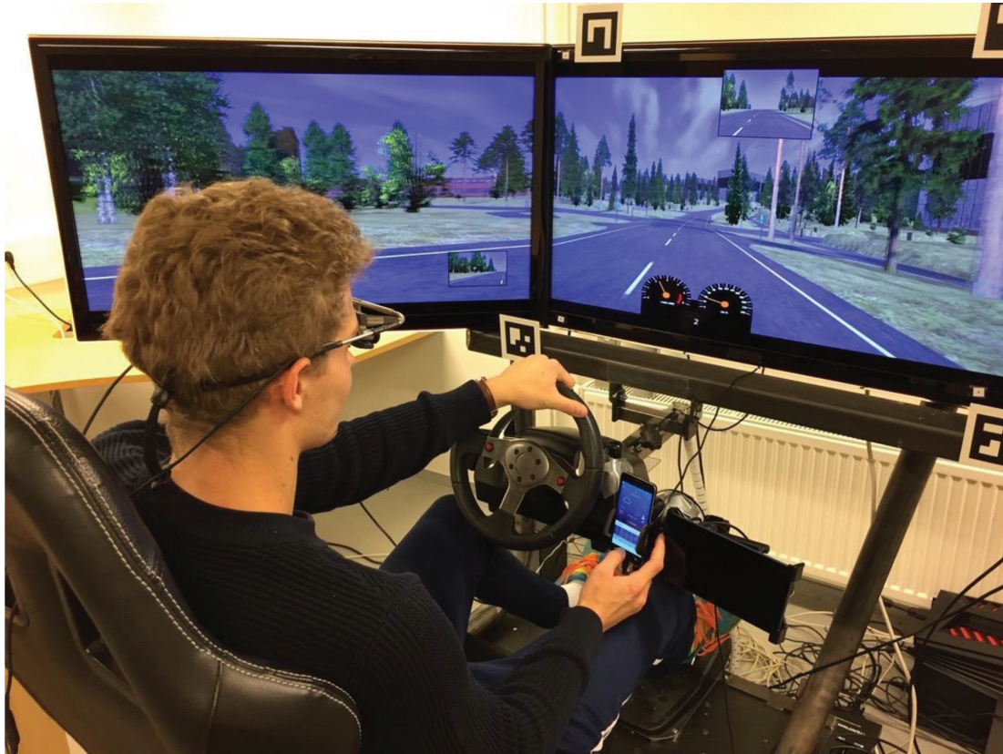
Figure 1. The experimental setup. The smartphone and the tablet are located next to the steering wheel. The participant is wearing a head-mounted eye-tracker.
