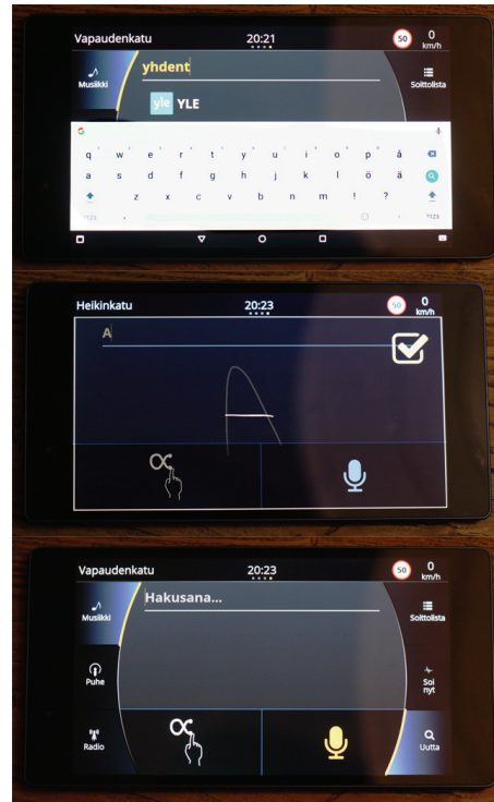
Figure 2: Three different text entry user interfaces: keyboard (on top), handwriting and voice recognition.
