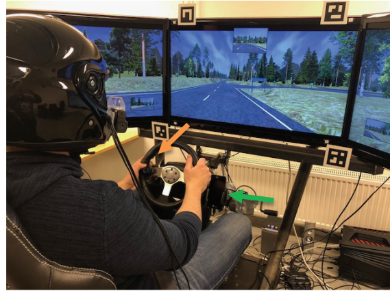
Figure 1: Experimental setup and the position of the devices. The orange arrow points to the steering wheel-mounted controller and the green arrow points to the smartphone.
