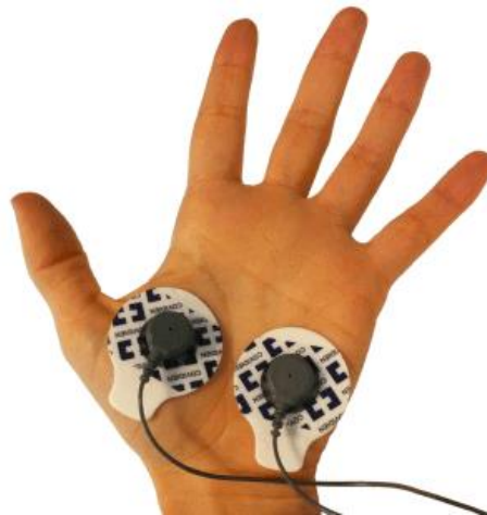
FIGURE 2A Electrodermal activity (EDA) electrode placement.
