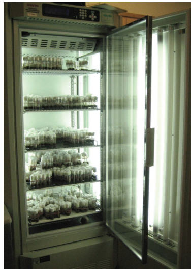
FIGURE 3 One of the environmental chambers used in the experiments (IV). In cases where there were many vials of flies in the chamber, the positions of the vials were changed regularly to allow the flies to experience as similar conditions as possible. (Photo: Tiina S. Salminen)
