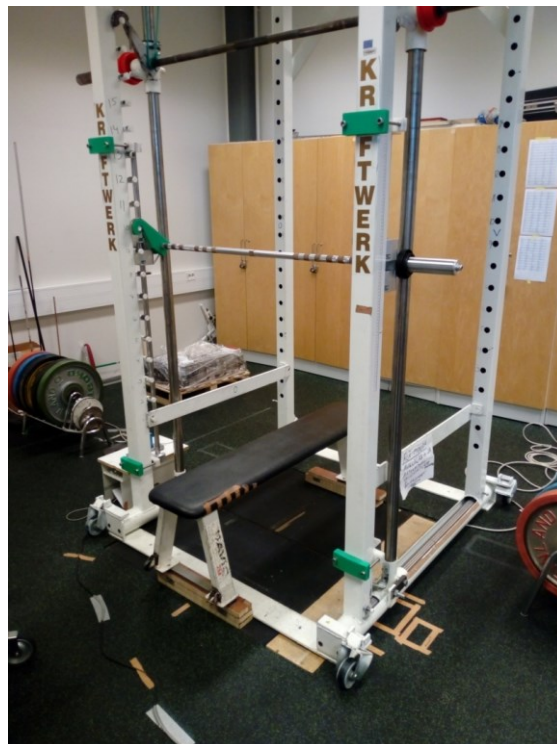
FIGURE 14. Customized Smith machine and force plate setting used to measure 1RM bench press and bench press throw performance.
