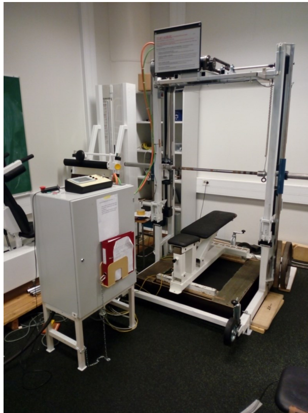
FIGURE 13. Custom-made isokinetic bench press device and the control panel.
