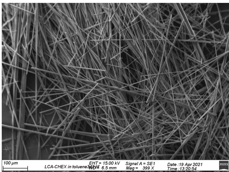
Figure 6. SEM micrograph presenting the fibrous gel network formed by lithocholic acid derivative as the gelator in toluene. R. Kuosmanen *et al.*, unpublished results.
