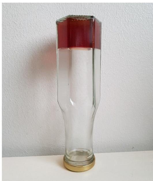
Figure 5. A polymer gel passing the ‘inversion test’.
