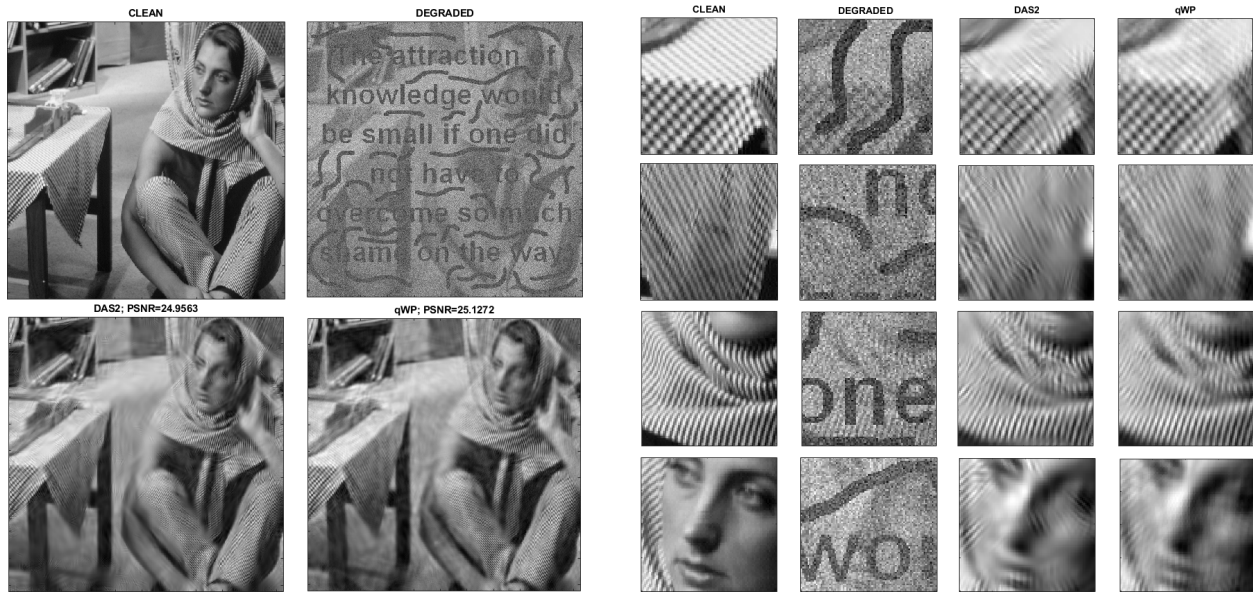
Figure 4.2: Restoration of “Barbara” image. Left: Top left: clean image. Top right: image degraded by application to it mask2 and Gaussian noise with \sigma = 50 dB. Bottom: Restoration by M2 (right), PSNR=25.13 dB, SSIM=0.4868 and by DAS-2 (left), PSNR=24.96 dB, SSIM=0.4709. Right: Fragments of images. Columns: First - clean fragments; Second – degraded; Third– restored by DAS-2; Fourth – restored by M2
