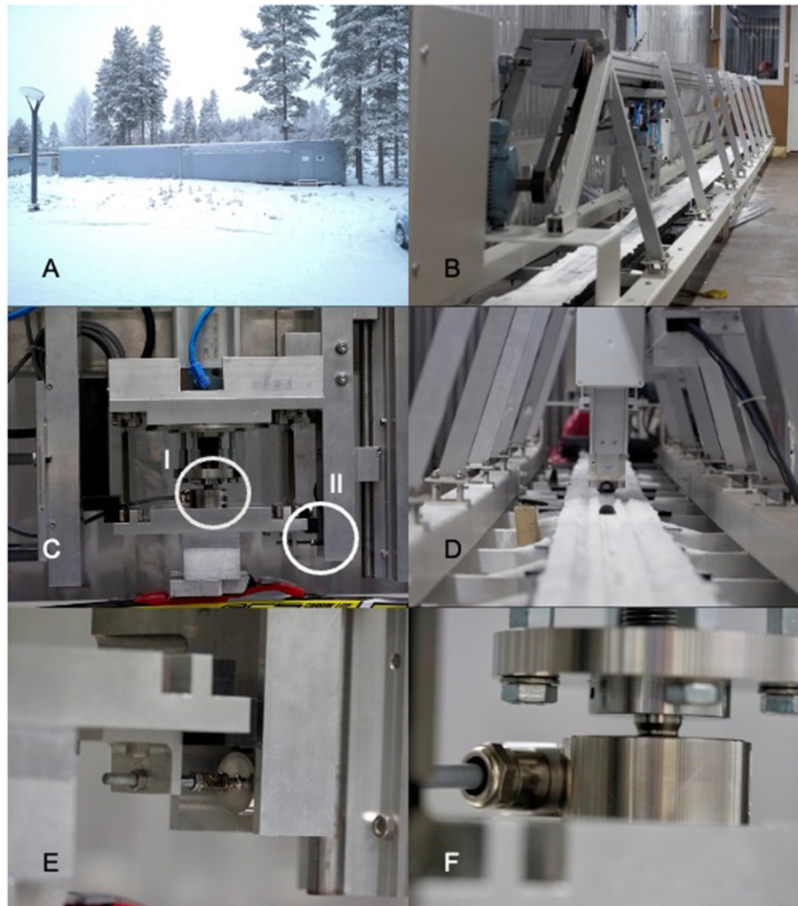
FIGURE 1 | (A) The laboratory is built of two 12 m long and 2.4 m wide insulated containers forming a 24 m long working space. The main section (21 m) is used as a low temperature laboratory and houses the skitester. A smaller (3 m) room at the end of the laboratory is used as an entrance and testing office/control room. (B) Frame of the skitester. The frame is 13.7 m long with an operating length of 10.81 m. Temperature can be set separately for the air and track (C) The skitester measurement unit has separate force sensors to measure vertical (I) and horizontal (II) forces. (D) Ski gliding on the testing track. (E) Closeup picture of horizontal sensor. Same as C(II). (F) Close up picture of vertical sensor. Same as C(I).
