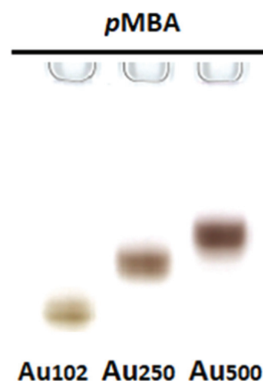
Figure 1. PAGE bands of Au102, Au250, and Au500 nanoclusters.
