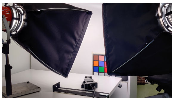
Figure 6. The used scanning setup: Two halogen lamps with a diffusor, color checker as an imaging target, and the hyperspectral imager, which was slid along the metallic ruler fixed to the desk.
