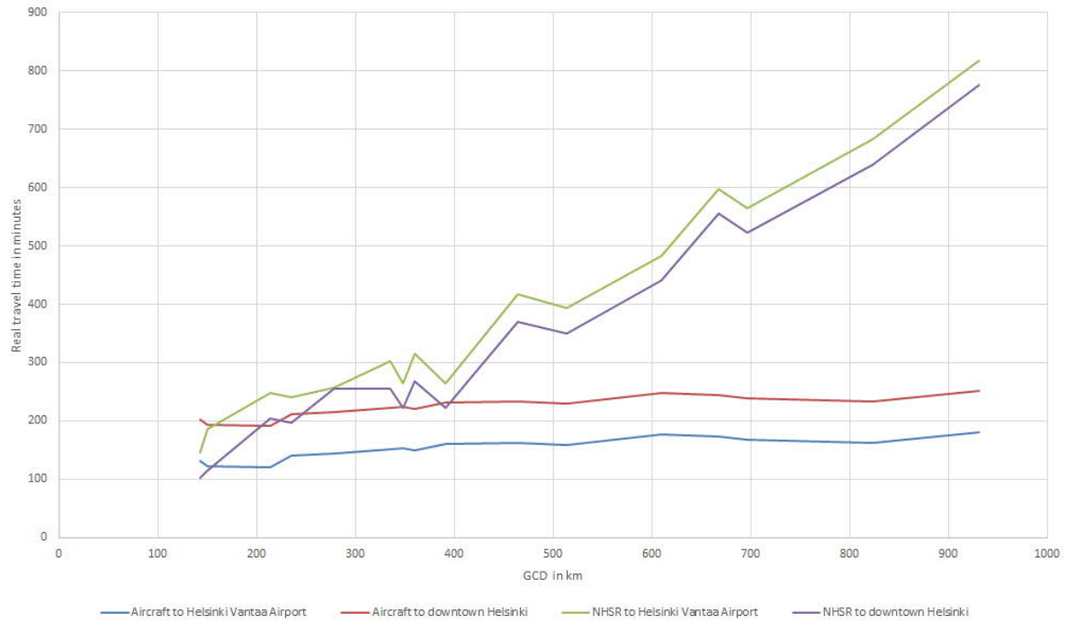
Fig. 6 Time-distance diagram for aircraft and NHR.
