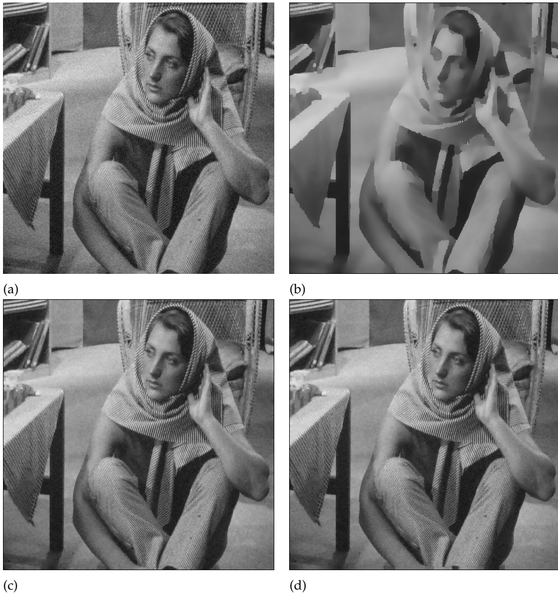
FIGURE 16 (a) Image with additive Gaussian noise \sigma = 12 . (b) Denoising using Felzenszwalb and Huttenlocher (2006). (c)-(d) Proposed method with span r = 1, 3 respectively.
