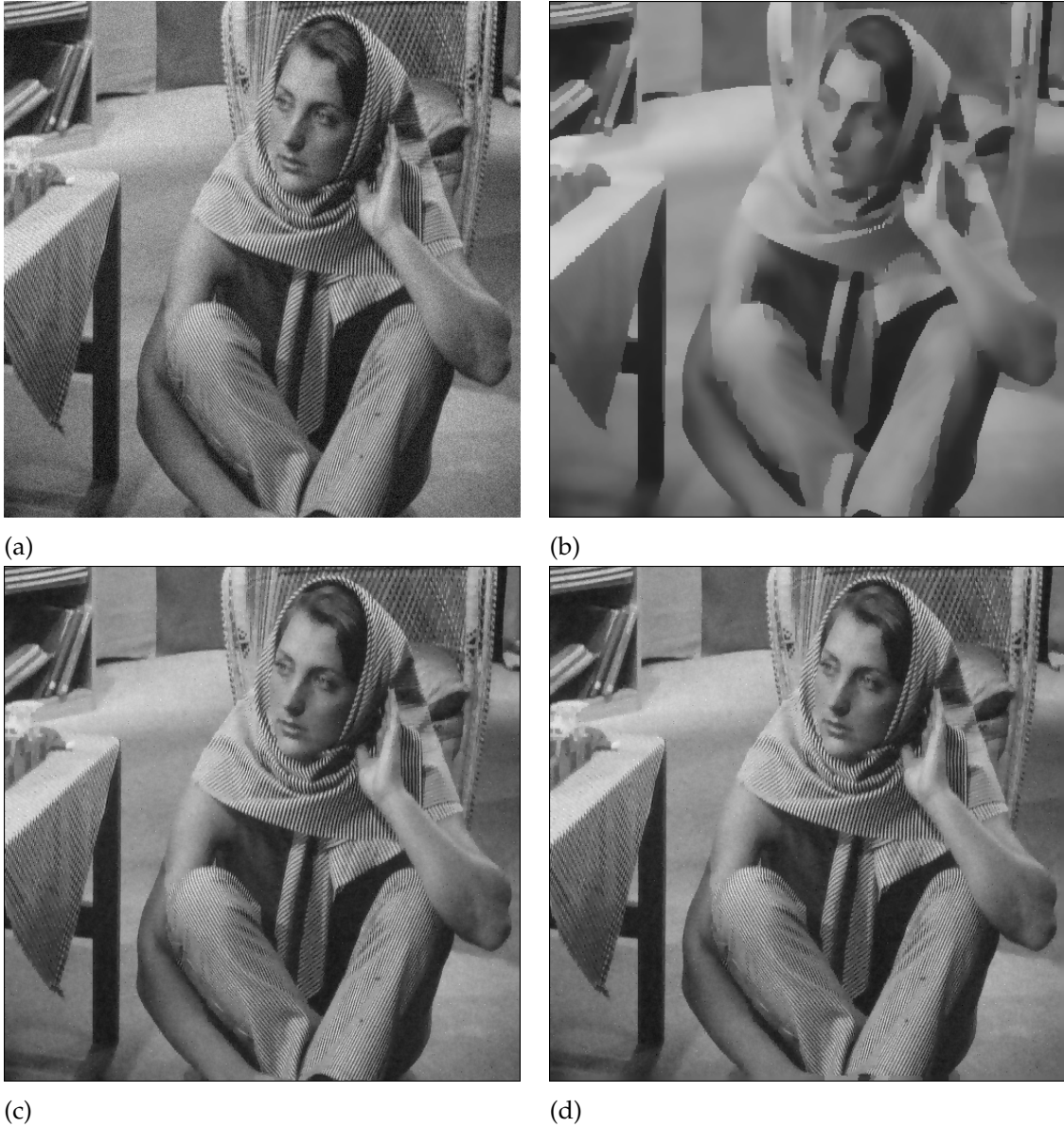
FIGURE 15 (a) Image with additive Gaussian noise \sigma = 10 . (b) Denoising using Felzenszwalb and Huttenlocher (2006). (c)-(d) Proposed method with span r = 1, 3 respectively.
