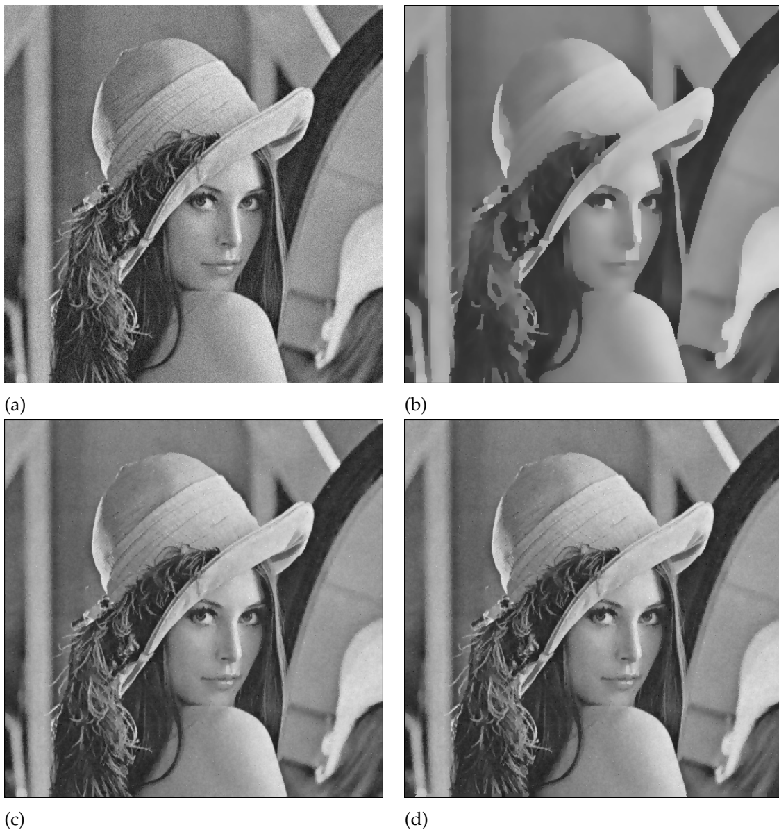
FIGURE 18 (a) Image with additive Gaussian noise \sigma = 10 . (b) Denoising using Felzenszwalb and Huttenlocher (2006). (c)-(d) Proposed method with span r = 1, 3 respectively.
