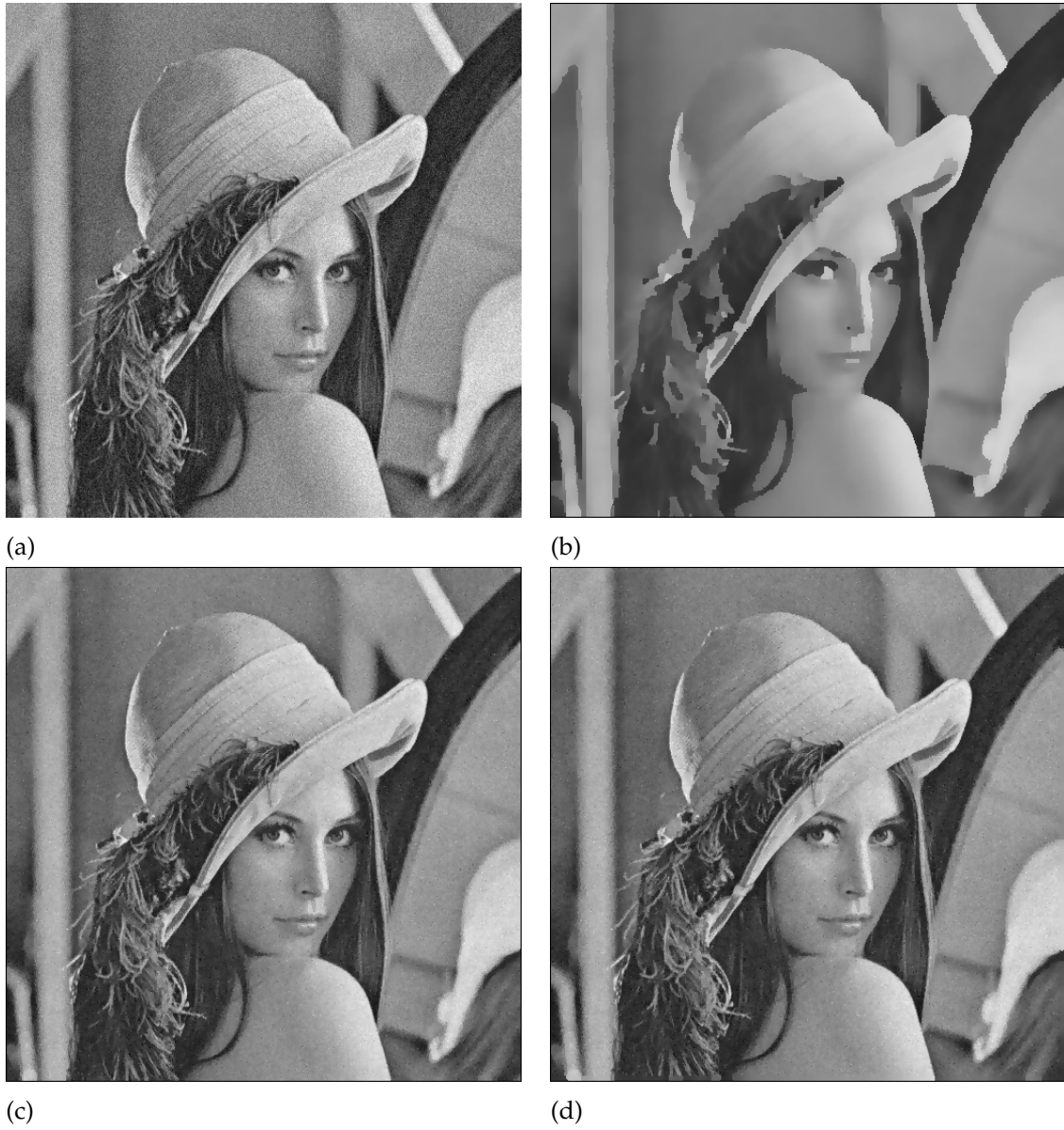
FIGURE 19 (a) Image with additive Gaussian noise \sigma = 15 . (b) Denoising using Felzenszwalb and Huttenlocher (2006). (c)-(d) Proposed method with span r = 1, 3 respectively.
