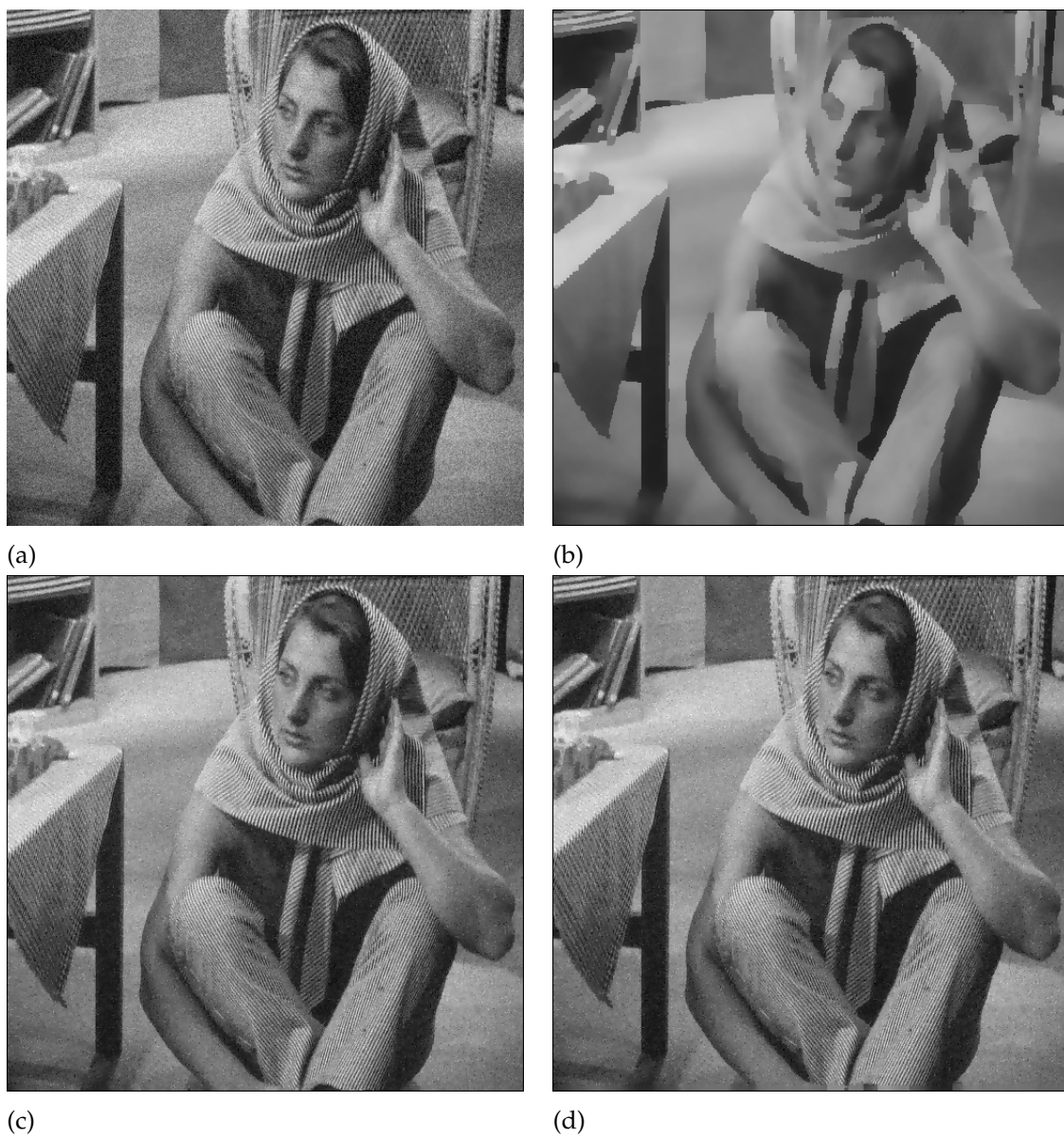
FIGURE 17 (a) Image with additive Gaussian noise \sigma = 15 . (b) Denoising using Felzenszwalb and Huttenlocher (2006). (c)-(d) Proposed method with span r = 1, 3 respectively.
