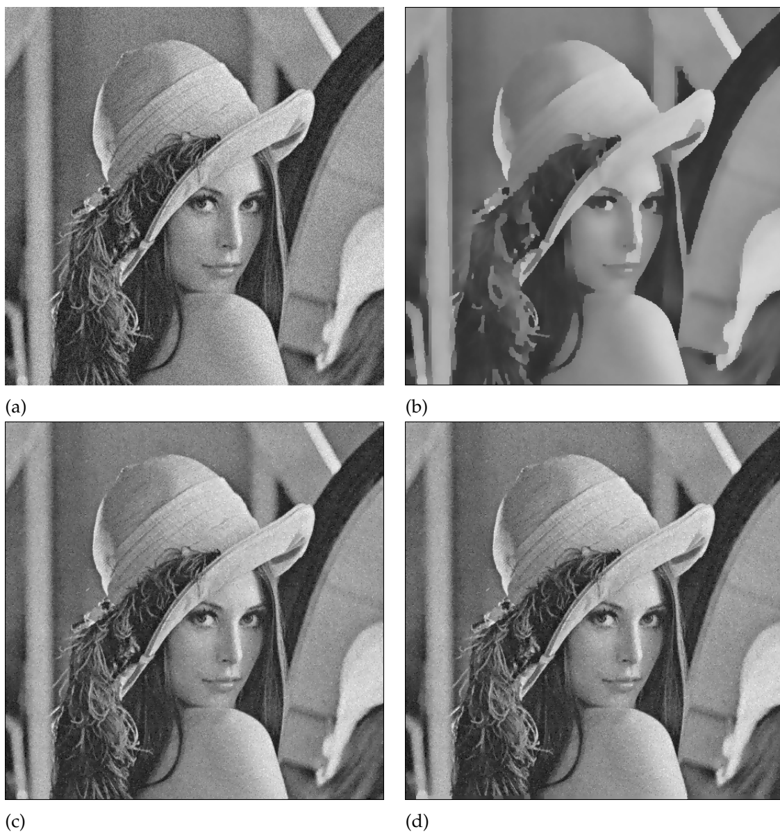
FIGURE 20 (a) Image with additive Gaussian noise \sigma = 15 . (b) Denoising Felzenszwalb and Huttenlocher (2006). (c)-(d) Proposed method with span r = 1, 3 respectively.
