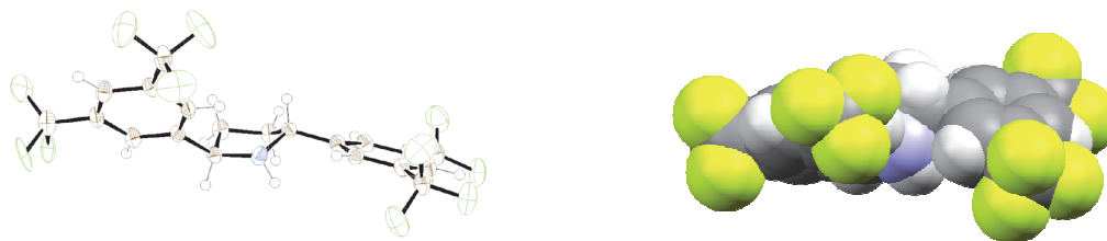
Figure 7: The X-ray structure of the catalyst ( R,R )- 31i . On the left, an ORTEP-presentation (ellipses with 50% probability), and on the right, a spacefill presentation (CSD-MULBED). 57,167
