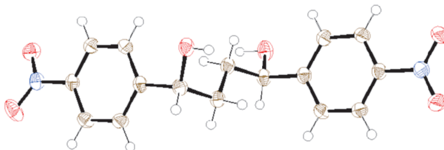
Figure 17: ORTEP-figure of the crystal structure of ( R,R )- 55d . Single crystal of the compound used in X-ray diffraction was obtained by slow evaporation of ( R,R )- 55d -solution in DCM-hexane. The thermal displacement parameters are shown at 50% probability level.
