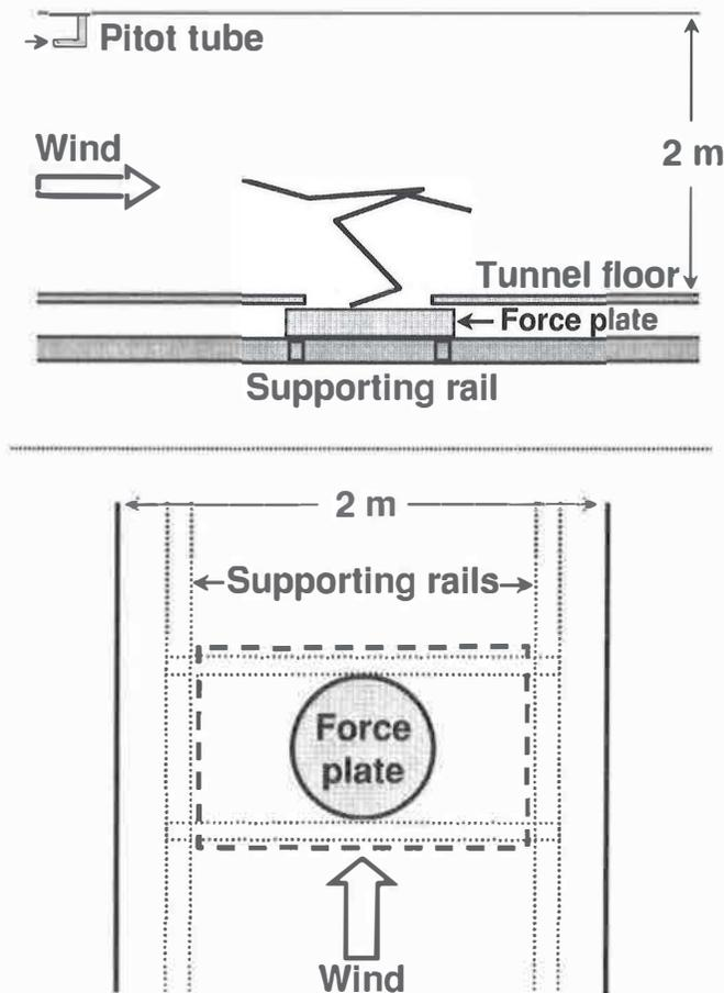
FIGURE 9 Schematic illustration of lateral (upper) and overhead (lower) views of the force plate arrangement in the wind tunnel.
