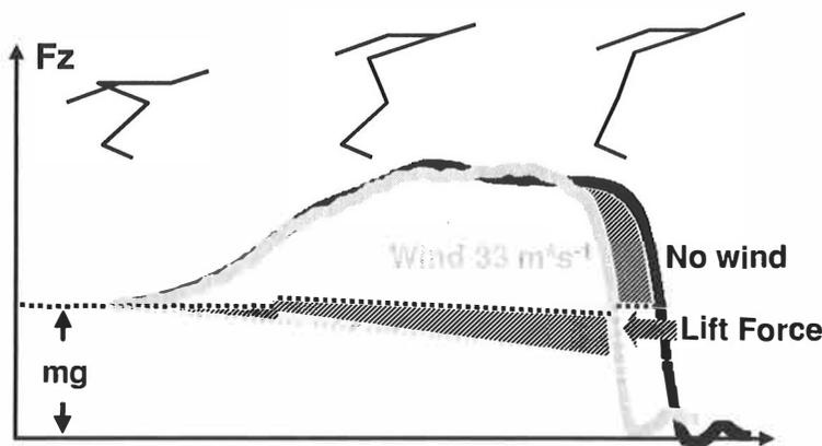
FIGURE 27 Schematic illustration of the possible behaviour of aerodynamic lift during ski jumping take-off.
