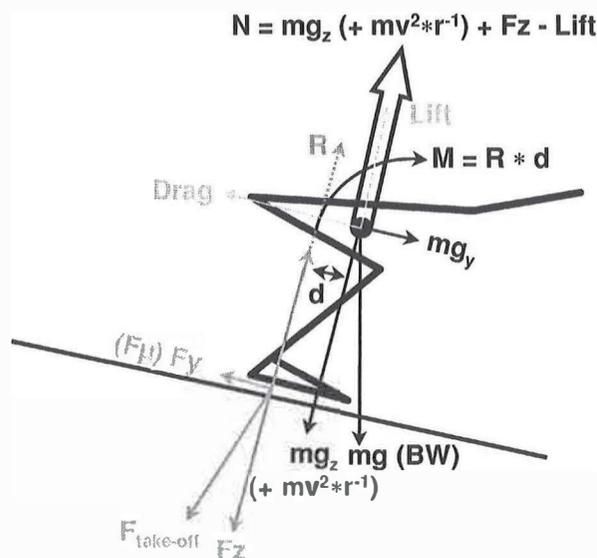
FIGURE 2 Forces acting on a ski jumper during take-off. To obtain maximum height the jumper's centre of mass (CM) should be located along the line of action of the vertical ground reaction force, whereas the production of angular momentum ( $M$ ) requires the CM to be located anterior to this line (Virmavirta 1999).
