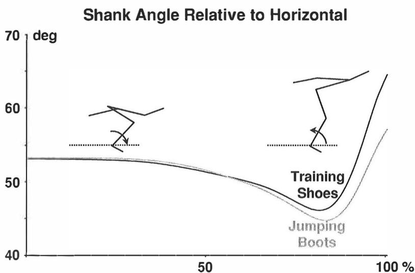
FIGURE 19 Time-normalised mean shank angle ( $n = 10$ ) during take-off, with training shoes and with ski jumping boots.
