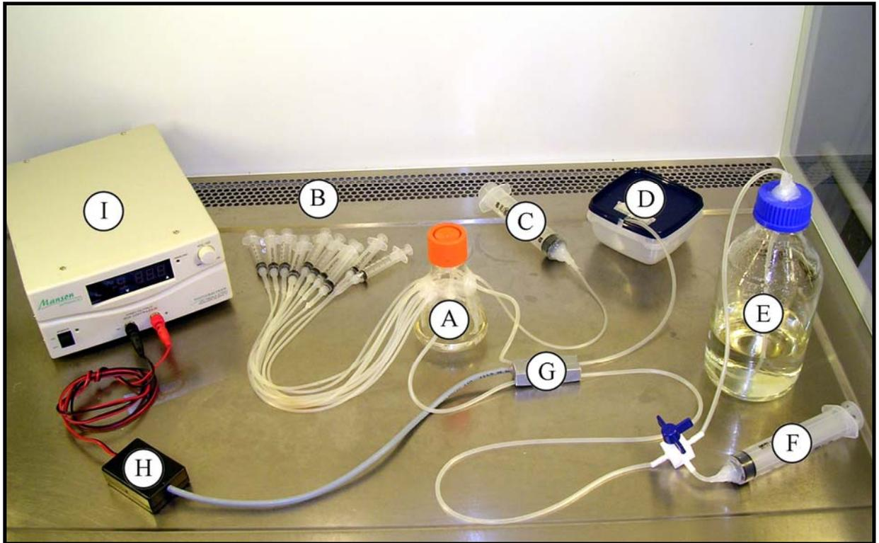
Figure 2. A: the microcosm, B: 10 sterile 5 ml syringes for sampling, C: a 50 ml storage syringe, D: Outflow tube submerged in 75 % alcohol, E: the resource stock bottle, F: a 50 ml syringe and 3-way valve for renewal of the resources, G: a heating element, H: a thermostat and I: a power supply for the heating element.
