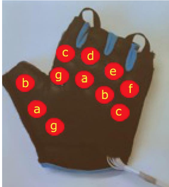
FIGURE 1. Fingerless KAIKU Glove with corresponding notes labeled on sensors.
