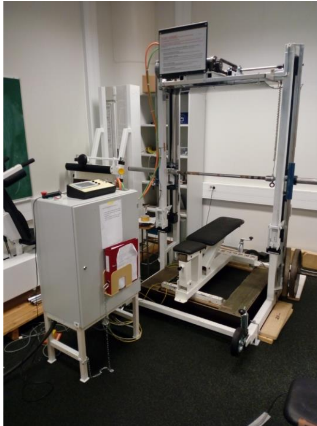
Figure 6. The custom-made isokinetic bench press machine with the operating panel positioned in front.
