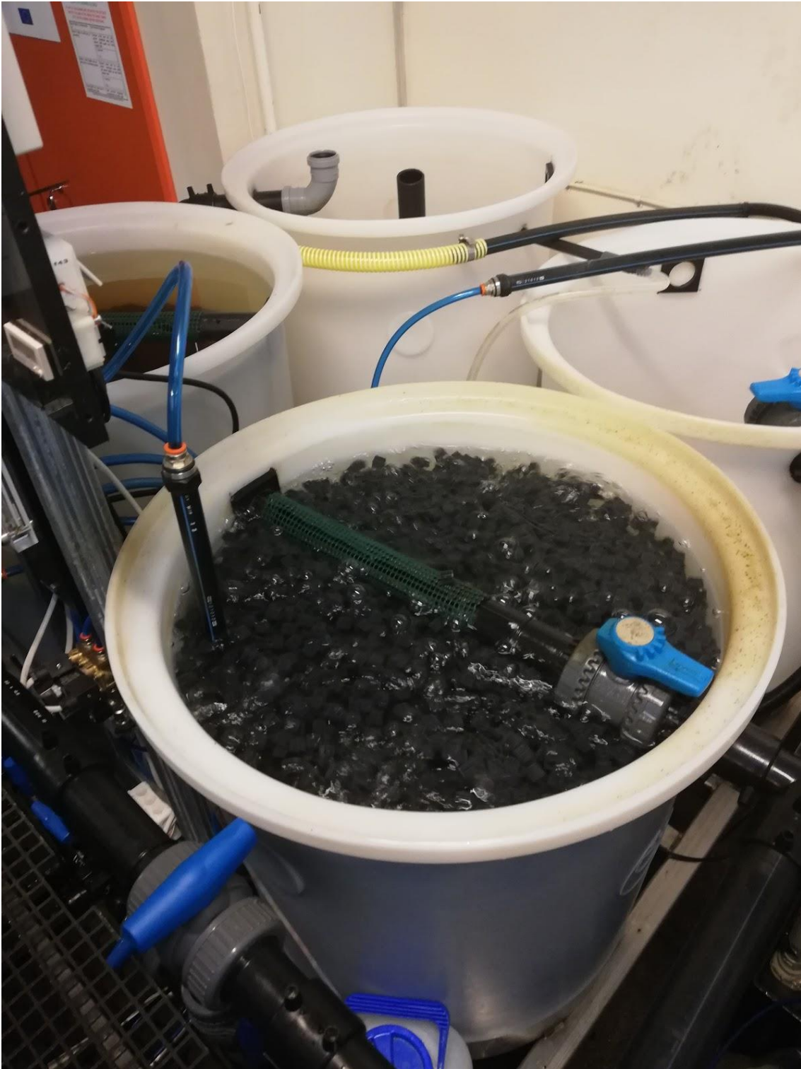
Moving-bed biofilter filled with constantly moving plastic media. On the left upper corner there is a fixed-bed biofilter, where the bioreactor water sample was taken.
