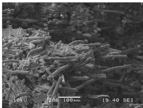
Figure 12. SEM micrograph of W_f = 40\% Tencel 1.7 dtex 3 mm composite fracture surface.
