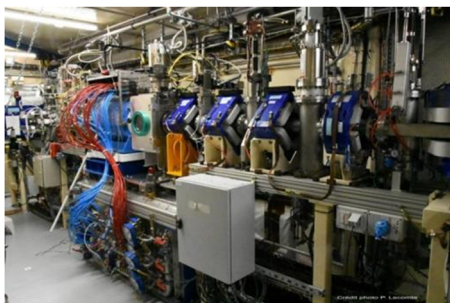
FIG. 2. Photo of the SP1 charge breeder installed in the middle of the LEBT.
