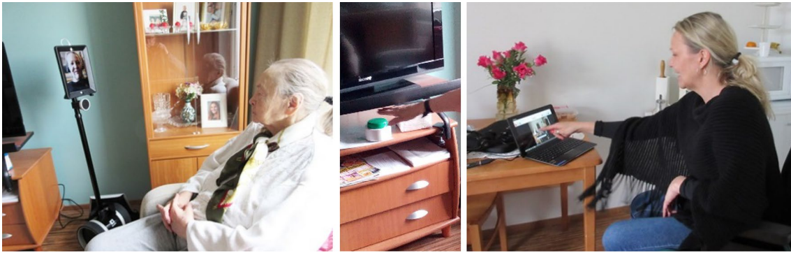
Fig. 1 The telepresence robot was placed in the room of the primary user in the care home (on the left). The resident could press a separate button to send an SMS request to her daughter to connect (in the middle). Her daughter used a laptop to connect with the resident (on the right)
