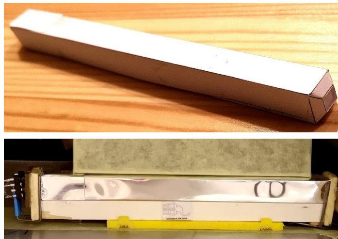
Figure 6.5: Enveloping of Scintillator 1 with paper and ESR foils.
