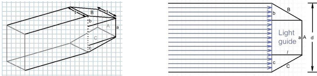
Figure 7.16: Schematic view of the scintillator with thickness matched to the photosensor size: 3D view of the geometry (left), 2D view of the parallel light entering the light guide (right).
