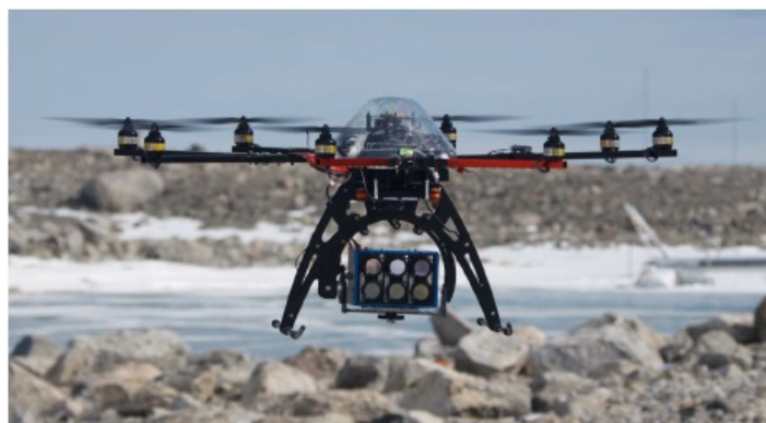
Figure 6. An OktoKopter UAV sporting a 6-band multispectral camera (Lucieer et al. 2012)
